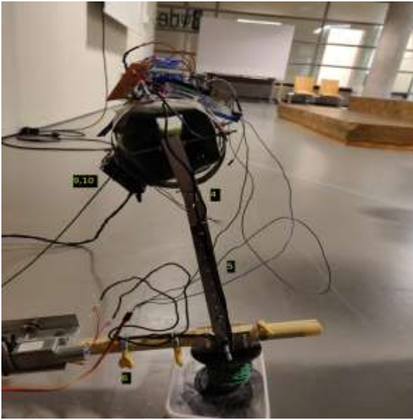
Figure 27 Frame of the arm; hose clamps (6), aluminum strips (5), hinge (4), batteries and battery holder (9,10)
