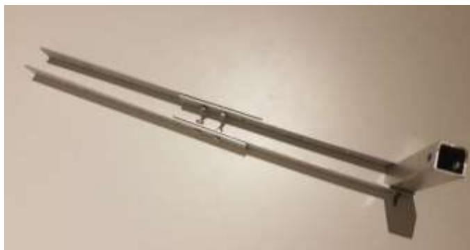
Figure 17 The adjustable under arm and the 'elbow'
