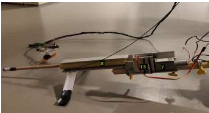
Figure 26 Shooting part; contains servomotor (13), dc motor (7) and spring (8)
