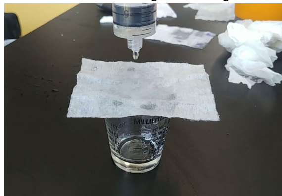
Figure 3. Setup of experiment 2. Water is squeezed onto the surface of the wicking fabric that is placed over a measuring container
