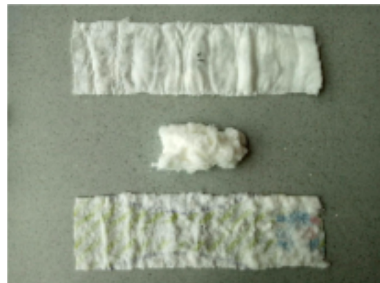
Figure 1. Separated layers of a diaper. Wicking layer (top), absorbent core (middle), and waterproof shell (bottom)
